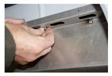
3. Slide the ash pan heat shield under the stove. Start the two sheet metal screws in the ash pan heat shield on the opposite end from the door. Do not fully tighten these screws yet. (It may be helpful to use a 2x4 on edge for support.)
